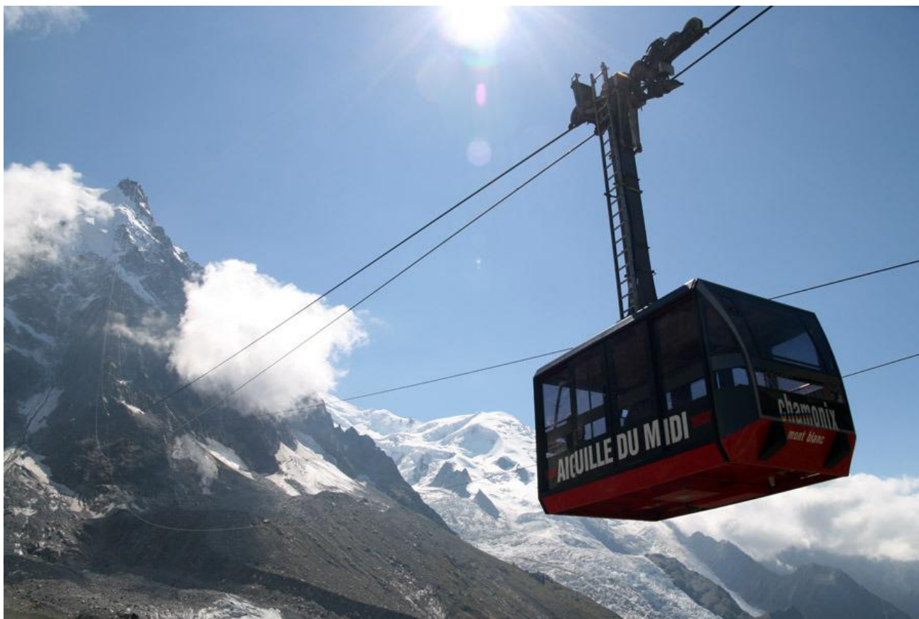
Figure 10: "Jigback Monocable System" Ropeway
