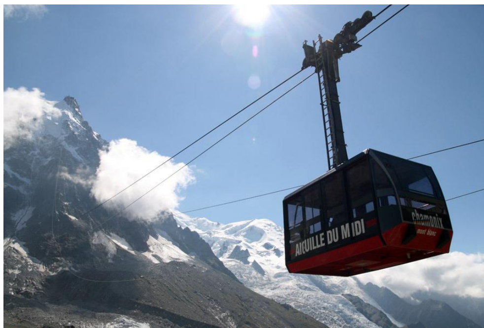
Figure 10: "Jigback Monocable System" Ropeway
